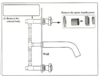
1.Drill the wall as the above drawing accrding, to the dimension of the fanucet. They are includes the main body conceal hole, cold water pipe hole, hot water pipe hole.
