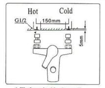
1.Fix hose inside the wall: The diamer of hose is G1/2.
